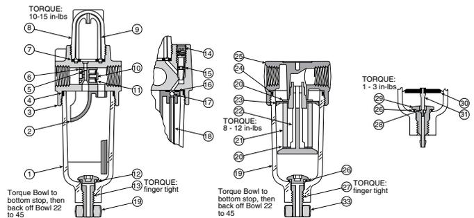
Figure 1: Micro-Mist Lubricator
