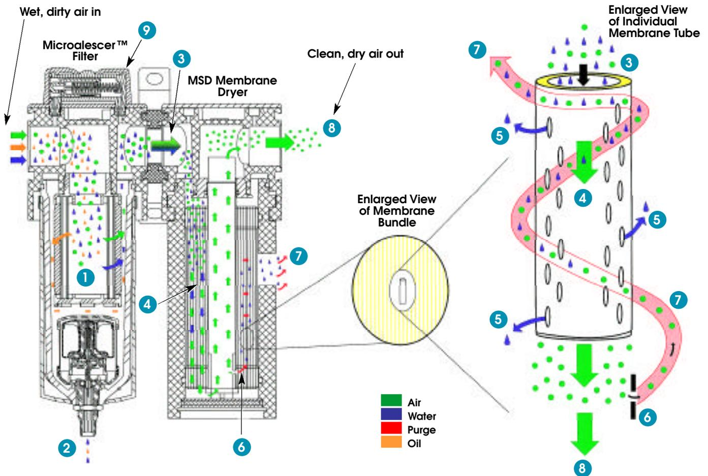
To achieve optimum performance and high quality compressed air for your application, it is imperative to install a Wilkerson Microalescer™ filter with automatic drain. The coalescing-filter prevents dirt particles and oil and water aerosols from contaminating the membrane. This drawing illustrates a typical clean, dry air system.
