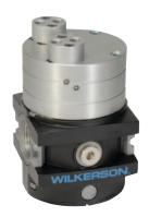
90 Series Combined Soft Start / Dump Valves, provide for the safe introduction of pressure to machines or systems. Soft Start / Dump Valves when set, allow the pressure to gradually build to the set point before fully opening to deliver full flow at line pressure.
